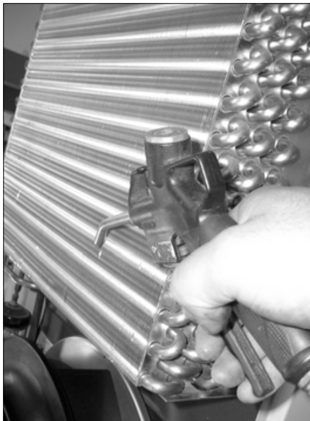
Fig. 56: Clean out the heat exchanger coil and compressor chamber using compressed air (1)
