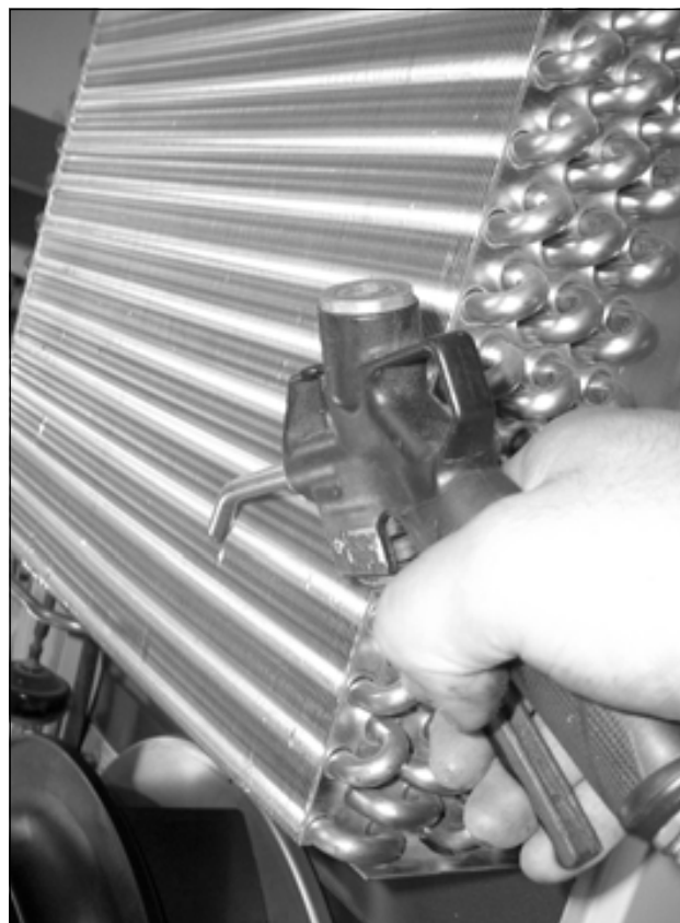
Fig. 80: Clean out the heat exchanger coil and compressor chamber using compressed air (2)
