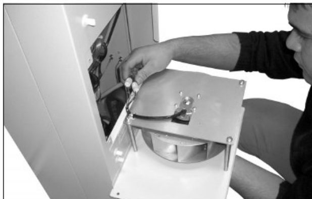
图69: 断开风扇接头 (1)
