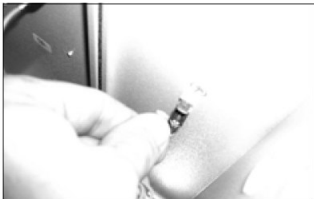
图73: 断开风扇接地电缆 (2)
