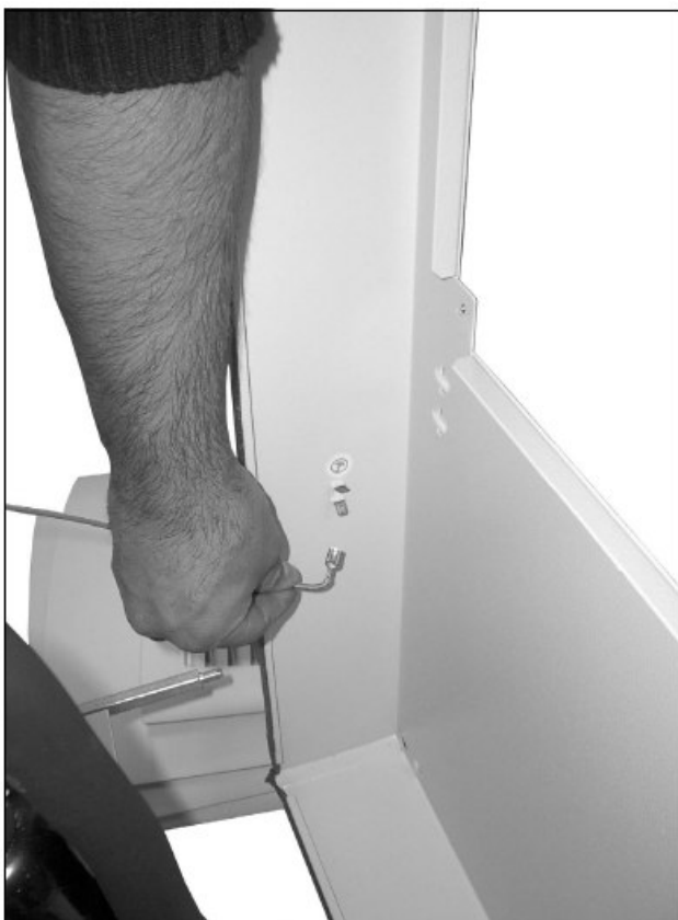
图77: 断开接地电缆 (2)
